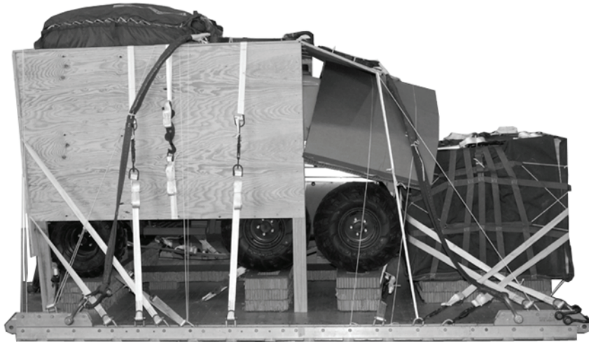
M-Gator with First Response Expeditionary (FRE) Fire Vehicle on a 12-Foot Platform
